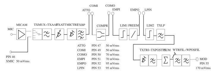
Signal levels are measured by oscilloscope and input signal frequency is 1 kHz. Transmitted signal deviation is 2.3 kHz.
