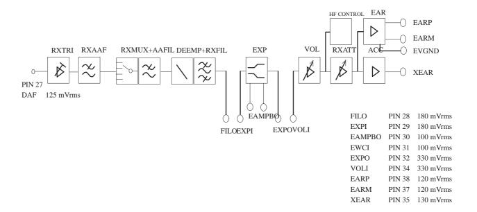
$Signal\ levels\ are\ measured\ by\ oscilloscope.\ Received\ signal\ audio\ frequency\ is\ 1\ kHz,\ deviation\ 5.7\ kHz\ and\ power\ level\ -53dBm.$
